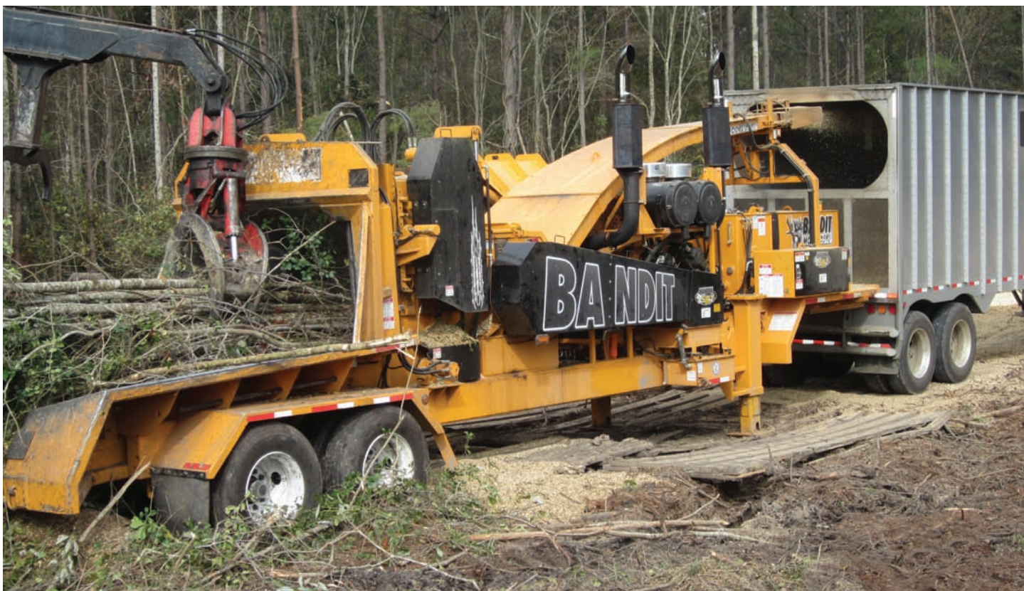
Cahoon Brothers Logging's Bandit Model 3590 micro-chipper. The Bandit is a towable, drum style whole tree chipper capable of producing more than 100 tons of chips in an hour. Models are available with 700 horse power and 875 horse power engines.
