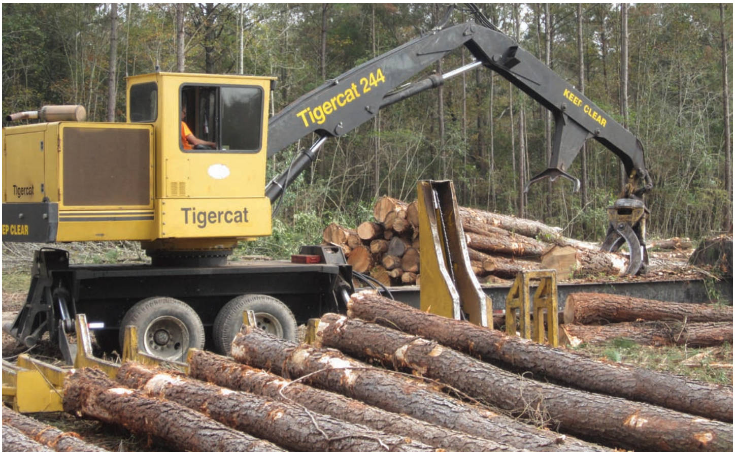
At the landing trees are processed and delimbed with Tigercat 234, 244 & 250 loaders all equipped with CSI delimbers.
